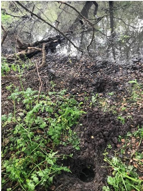
Photo 11. Soil test pit one excavated as part of the jurisdictional delineation.
